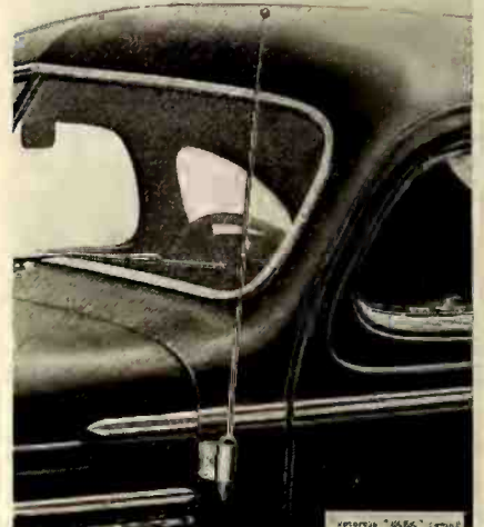
Motorola's new "Rocket" aerial which requires no drilling of holes, being mounted inside the hood of the car.
